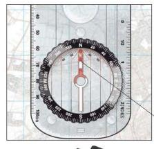
Keeping orienting lines 2 aligned with the grid lines on the map, rotate the entire map until the north magnetic needle on the compass sits inside the orienting arrow. The map is now set to magnetic north and should basically line up with the features that surround you.
