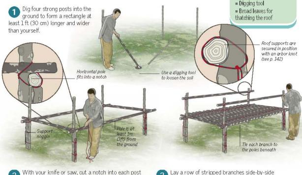
With your knife or saw, cut a notch into each post deep enough to fit the curve of the horizontal pole.
