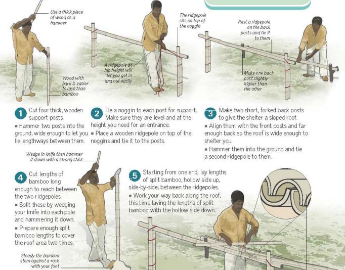
The split bamboo \_ layers of the roof direct water into the gutter
