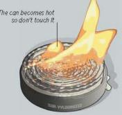
When the can has cooled down, hold it at an angle and light the top of the cardboard with the candle. The flame should be concentrated and spread across the top of the can.
