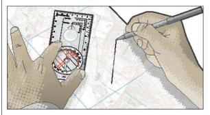
TRANSFERRING THE BEARING ONTO THE MAP Place the top left corner of the compass base plate over the feature on your map. Keeping it there, rotate the entire compass until the orienting lines are parallel with the vertical grid lines. Draw a line from the feature down the left side of the base plate to map your bearing.
