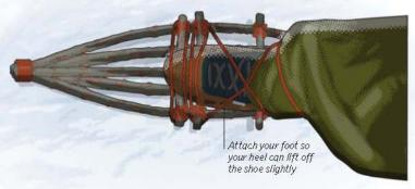
Place your foot on top of the snow shoe, ensuring that the ball of your foot sits directly over the front cross-piece and that your heel is positioned on the back cross-piece.
