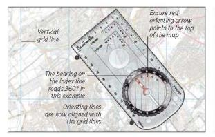
Turn the compass housing around until the orienting arrow and the orienting lines within the housing line up with the vertical grid lines on the map. Read the bearing between the two points from the index line on the compass.
