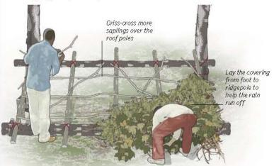
Apply the covering to the woven skeleton of the roof and walls.
