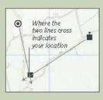
Using your compass, take bearings to the features on the ground.
