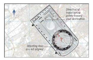
Lay your map on a flat surface, ensuring that there's nothing nearby to interfere with the compass reading (see box, p. 69).
