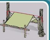
HAMMOCK AND TARP Tie a ridgeline above the hammock. Drape the tarp over the line and anchor it on either side to a horizontal pole tied to two uprights.
