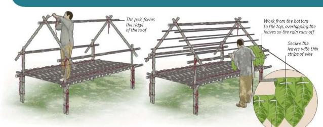
Tie poles together to form two A-frames. Tie these on top of the roof support poles at each end of the framework.
