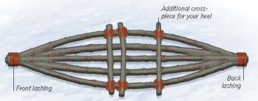
2 Lash the five loose lengths of wood together at the back of the shoe. It's important to make this lashing as secure as possible.
